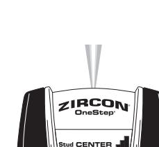
Continue sliding tool. When the center of a stud is located with three bars on the Signal Strength Indicator, the four Middle bars, CENTER display, and SpotLite® Pointing System will all illuminate and the buzzer will sound.
