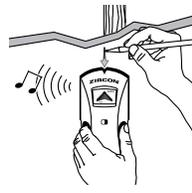
Without releasing Power button, continue scanning beyond marked spot until some segments of the arrow turn off. Slide unit in reverse direction to locate other edge of stud.
