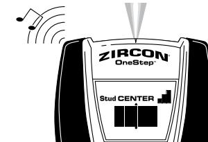
In cases of deeper studs (thicker walls) when the center of the stud is located only two bars will show on the Signal Strength Indicator and only the SpotLite® beam and four Middle bars will illuminate. If you still can't locate a stud, try the next step.
