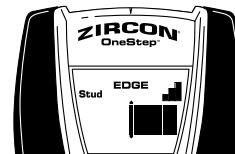
Continue sliding tool. When the center of stud is located with three bars on the Signal Strength Indicator, the four Middle bars, CENTER indication, and SpotLite® Pointing System will all illuminate, and the buzzer will sound.
