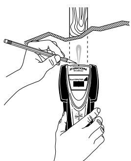
**! WARNING** Electrical field locators may not detect live AC wires if wires are more than 2 in. (51 mm) from the scanned surface, encased in conduit, present behind a plywood shear wall or metallic wall covering, or if moisture is present in the environment or scanned surface.
