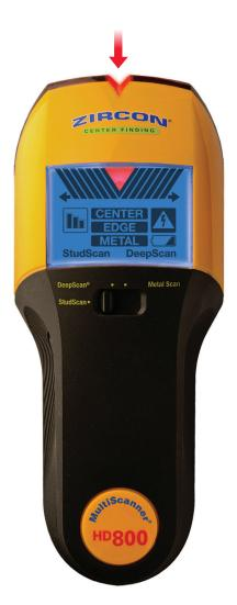
MultiScanner<sup>®</sup> HD800 quickly and easily locates the center and edges of wood and metal studs and joists behind walls, floors, and ceilings. It also locates metal targets up to 3 in. (76 mm) deep. A 3-mode switch makes it easy to change functions, while the backlit display screen, SpotLite<sup>®</sup> Pointer, and audio tone all indicate the location of the target.
