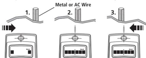
In METAL SCAN mode, if you calibrate directly over metal, you likely will not detect any metal. Move tool a few inches left or right, release the Power Button, and start over.
