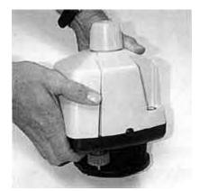
Pull firmly on tab at base of door to remove.
