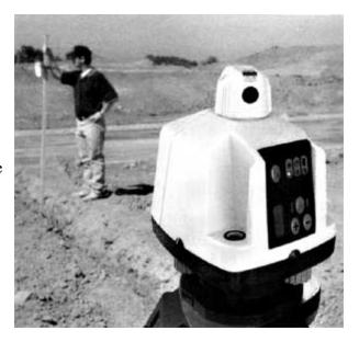
If long distance is required, the LaserVision® AUTO can be set-up in the middle of a site, covering a total diameter of 1,000 feet (300 meters) using an optional receiver.
