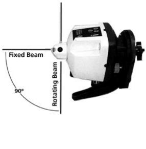
When the LaserVision® AUTO is in vertical mode, it is completely manual in operation and will not turn off if it is disturbed. Check the vertical vial and your benchmarks regularly to be sure your work will be accurate. The LaserVision® AUTO is designed for vertical alignment up to two stories high.
