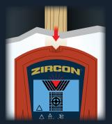
Continue sliding. When target center is detected, target icon displays and SpotLite® Pointer illuminates. Mark this location.
