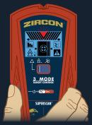
Always start your wood stud scan in Target Control™ (TC™) mode. Move mode selector switch to left. Place scanner flat against wall. Press and hold Power Button. Wait for beep.
