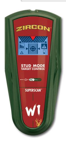
Featuring new, revolutionary Target Control™ (TC™) Level 1 Technology. The Zircon® SuperScan™ W1 advanced stud finder is tuned to find clean, wood studs while filtering out metallic false positive objects, such as plumbing, conduit, straps, brackets, or ducts, hidden behind surfaces. The LoLevel™ Indicator signals to the presence of dangerous, deep, and less dense false positive targets, reducing the chance of accidentally drilling into objects such as plastic pipes.
